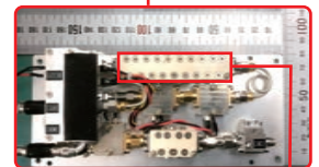
16-24GHz Analog module Isolator / Amplifier / Anti-aliasing filter
